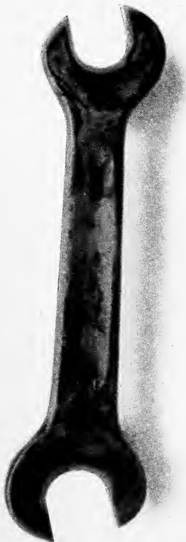
Fig. 3. Reproduction of Wrench showing Effects obtained by Methods for Casehardening and Coloring described in Chapter V.
